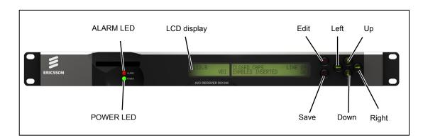
Figure 3.2 Front Panel Controls and Pushbuttons
